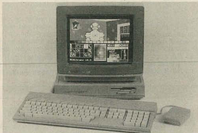
FIG. 3—ATARI'S MEGA 4 includes four megabytes of RAM, an 8-MHz 68000, 3.5" floppy-disk drive, and the GEM operating system.
